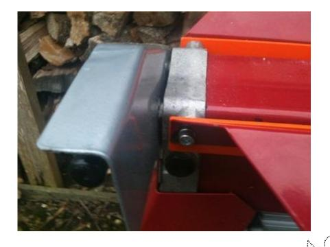
5. Ram Stop Rails in situ showing slot close to the log pusher, stopper plate is installed in this photograph
