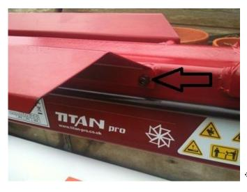
3. Remove the back bolt from side wing and washers supplied)
