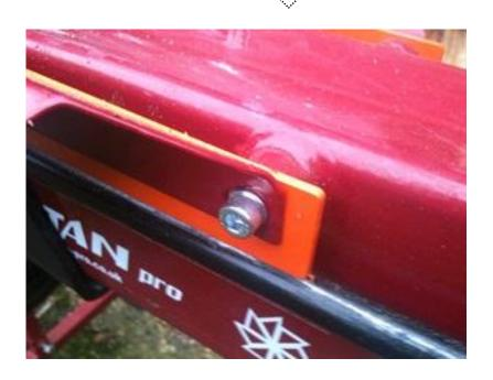
4. Install horizontal rails between the side wing and the body of the machine. Use all **new** bolts and washers supplied
